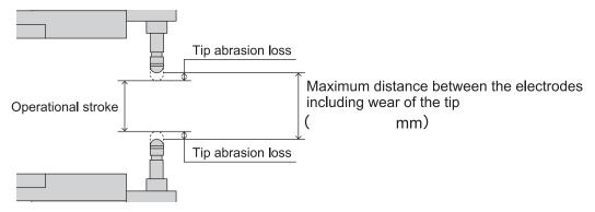
8) The whole stroke length of the welder pressure cylinder
