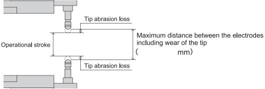
8) The whole stroke length of the welder pressure cylinder
